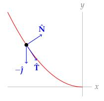
Let  $W\hat{\mathbf{N}}$  be the normal force exerted by the wire when the bead is at position x. Note W > 0. Is  $\frac{dW}{dx}$  positive or negative?
