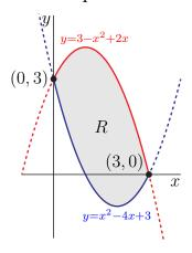
Note that the curves  $y = x^2 - 4x + 3$  and  $y = 3 - x^2 + 2x$  intersect when  $x^2 - 4x + 3 = 3 - x^2 + 2x$  or  $2x^2 - 6x = 2x(x - 3) = 0$  or x = 0, 3.
