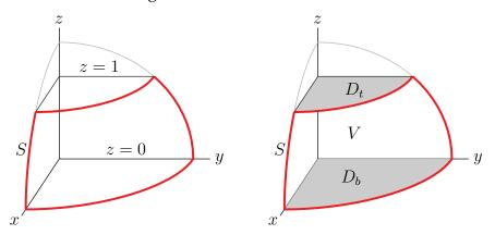
The surface *S* is not closed, and so is not the boundary of a solid, so we cannot apply the divergence theorem directly. But we can easily come up with a solid whose boundary contains *S*. Let
