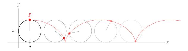
A circle of radius a rolls along the x-axis in the positive direction, starting with its centre at (a, a). In that position, we mark the topmost point on the circle P. As the circle moves, P moves with it. Let  $\theta$  be the angle the circle has rolled — see the diagram below.
