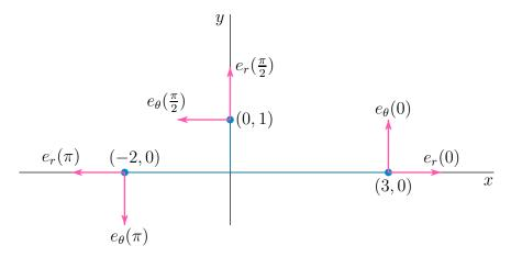
and here is a sketch (to a different scale) of  $(x_i, y_i)$ ,  $\hat{\mathbf{e}}_r(\theta_i)$ ,  $\hat{\mathbf{e}}_\theta(\theta_i)$  for i = 2, 4 (the points off the axes).
