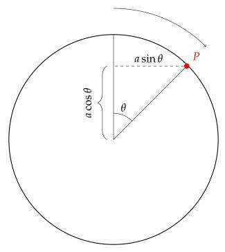
From the diagram, we see that *P* is  $a \cos \theta$  units above the centre of the circle, and  $a \sin \theta$  units to the right of it. So, the position of *P* is  $(a + a\theta + a \sin \theta, a + a \cos \theta)$ .
